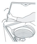
Fig.19 Removing the lid
